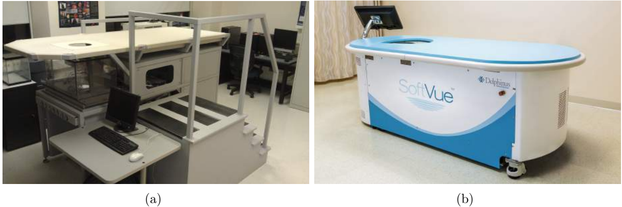
Figure 5.1: Ultrasound Tomography Devices. (a) CURE. (b) SoftVue.
